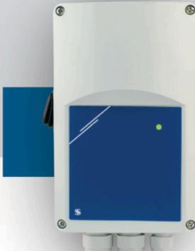
The EVS-1-XX-DM electronic speed controllers automatically control the speed of single-phase voltage controllable electric motors (230 VAC / 50–60 Hz). These units are equipped with Modbus RTU communication and provide a wide range of functionalities: remote control options, adjustable off level, min. and max. output voltage settings, and time-limited motor operation initiated by a logic or switch signal.
